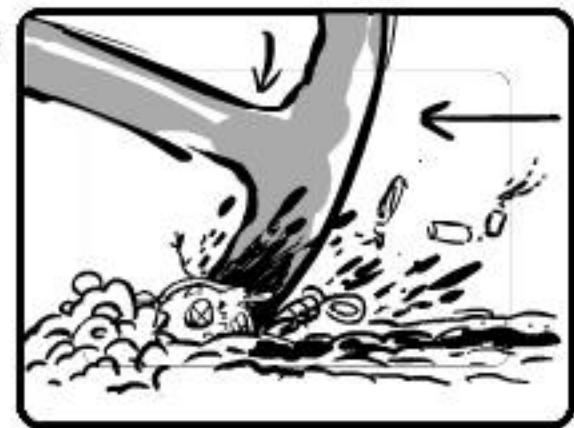
Anchor is digging deeper and is slowing down
